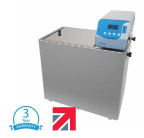
This Deep Chamber Bath<sup>™</sup> is suitable for Gerber testing or where deeper water volumes are required.
