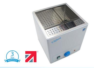
Unstirred Clifton DeepChamberBath™, with Thermostatic analogue control provides a deep volume of temperature controlled water. Comprising of a stainless steel tank housed in a durable paint finished outer case. Painted surfaces feature a tough anti-bacterial finish with good chemical resistance. Complete with a removable stainless steel perforated shelf.
