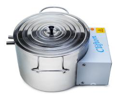
Constant level device maintains liquid level during boiling. Use standard laboratory tubing and connect one outlet to a tap and adjust the water supply to maintain boiling water level. The other outlet acts as an overflow to a sink or drain.
